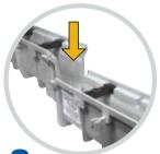
2 Slide second Dura Slope™ section into place
