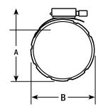
Installed Dimensions A and B
