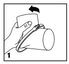
Rotate fitting to desired angle.
