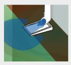
Downspout Aprons don't move water far enough away from foundations and can add to erosion and flooding
