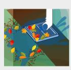
Flat Grates cause splashing, can clog with debris and heavy-flows often overshoot the grate
