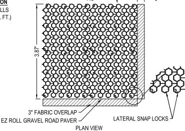
GRAVEL INFILL LEVEL ADJOINING FINISH GRADE EZ ROLL GRAVEL ROAD PAVER 1/4" to 1/2" PAVER GRIDWORK -FINISH GRADE **GRAVEL INFILL -**RECOMMENDATIONS: CLEAN, WASHED 1/2" AASHTO #57 BASE ROCK OR OTHER APPROVED MINUS STONE EQUAL AS SPECIFIED BY PROJECT ENGINEER COMPACT NATIVE SOILS
