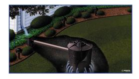
**Pop-Up Emitter** – Acting as the discharge point of a drainage system, Pop-Up Emitters release water from the drain pipe away from structural foundations in order to help manage water overflow. A spring-loaded cap opens when it senses the hydrostatic pressure of water flowing through the pipe, and it closes again when the flow decreases. The pop-up style keeps rodents and debris out of the system, and the low-rise height won't get in the way of mowers.
