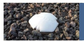
Used with EZ Roll™ Grass and Gravel Pavers, NDS EZ Marker™ is a modular solution to outlining driving lanes, parking stalls, and fire lanes. After the pavers have been unrolled, pinned, and secured, EZ Marker™ snaps into the appropriate empty cells to outline whatever pattern necessary to properly direct vehicular traffic.
