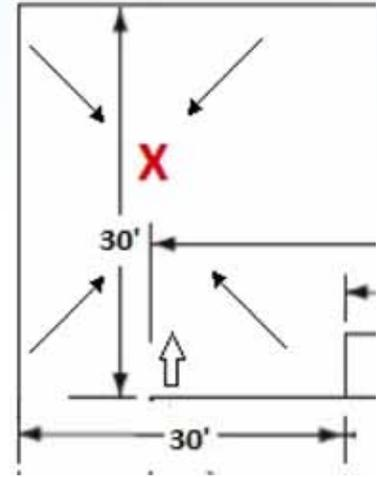
We can now determine the drainage zones. Each area where the arrows point to is a separate drainage zone. Multiple parts of your property may drain to a single drainage zone. In our example property, the back-left portion of the roof and the back-left portion of the lawn drain to "X". Labeling and coloring each drainage zone helps keep everything clear. The picture below shows drainage "Zone A". Notice that everything that drains to this zone is colored yellow.
