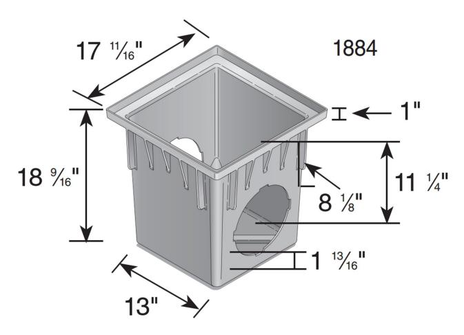
Material: UV Protected High Density Polyethylene (HDPE)
