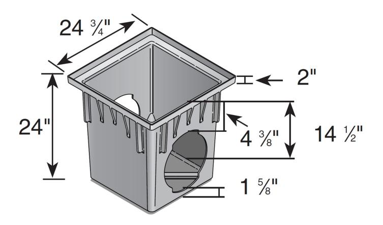
Part #: 2400 ( 2 Openings) and #2404 ( 4 Openings) Material: HDPE (High Density Polyethylene) Color: Black Use with 24" x 24" Grates Fits: 3" or 4" Sch. 40, sewer, drain, corrugated, and triple wall pipe, 6" and 8" sewer, drain and corrugated pipe, 10" and 12" sewer, drain and dual wall corrugated pipe, 12" single wall corrugated pipe will not fit 10" single wall corrugated pipe. Requires 2 or 4 #2410 Universal Outlet
