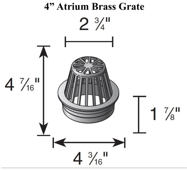
Part #: 78B Material: Brass Color: Bass Fits: 4" sewer, drain, pipe & fittings, 4" corrugated & triple wall pipe. Grate Opening: 1/4" Open Surface Area: 10.2 Sq. Inches Head Pressure / Flow Rate: Head (inches) - Max Flow 1.0" = 44.13 GPM0.5" = 31.2 GPM Weight Per Each: 2.0 lbs.
