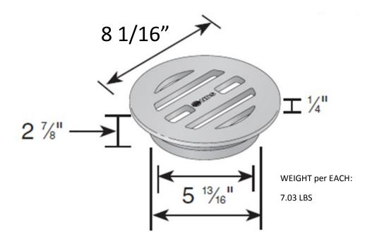
Material: Ductile Iron Colors: Black (D6) Fits: NDS Spee-D Basin, 6" Corrugated and Sewer and Drain pipe. This is not a custom grate and qualifies for normal NDS freight terms. Opening: 7.05 in<sup>2</sup> open space Will accommodate 21.57 gallons per minute with 1/2" of head
