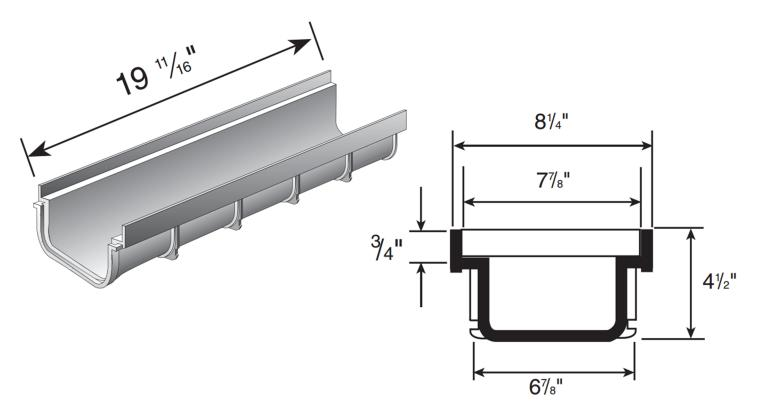
Material: UV Protected PVC Colors: Gray (830) Weight: 2.00 lbs each Interlocks with other Shallow Profile 8" Pro Series Channels. Should be installed a minimum 1/8" below finished grade for non-traffic applications and 1/4" below finished grade for traffic applications. Grate sold separately.
