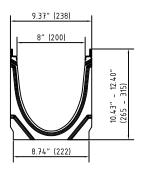
**MATERIALS:** Channels shall be manufactured from Filcoten fiber composite with concrete edge cast galvanized rail. Minimum properties of Filcoten fiber composite will be as follows:
