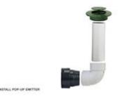
Using a Corrugated Pipe Adapter, connect the EZ-Drain to an elbow with a weep hole. The elbow should be installed with the weep hole on the horizontal side of the elbow. Slide the Pop-up Emitter onto the elbow. An additional length of pipe can be used to bring Pop-up emitter to the surface.
