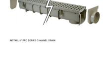
follow installation instructions included with the channel when installing the channel drain. The 5" Pro Series Channel Drain should be installed a minimum of 1/4" below the finished grade of the surrounding surface. Connect the required number of channel sections together using interlocking end connections. Place the grates on the channel and screw in place. Installend caps at the end of the runs as needed. Step 3: Connect elbow to drain on channel
