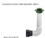
Connect the drain pipe to an elbow with a weep hole. The elbow should be installed with the weep hole on the horizontal side of the elbow. Slide the Pop-up Emitter onto the elbow. An additional length of pipe can be used between the elbow and Pop-Up Emitter to bring the Pop-up emitter to the surface. The Pop-Up Emitter fits on the "bell" or "hub" end of the pipe or a pipe coupler.
