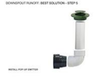
Using a Corrugated Pipe Adapter, connect the EZ-Drain to an elbow with a weep hole. The elbow should be installed with the weep hole on the horizontal side of the elbow. Slide the Pop-up Emitter onto the elbow. An additional length of pipe can be used between the elbow and Pop-Up Emitter to bring the Pop-up emitter to the surface. The Pop-Up Emitter fits on the "bell" or "hub" end of the pipe or a pipe coupler.
