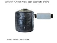
The Flo-Well should be installed in a low spot in your yard. Knock out the appropriate holes in the side panels of the Flo-Well where the EZ-Drain will be installed. Assemble the Flo-Well using the interlocking side panels. Slide the EZ-Drain through the hole in the Flo-Well side panel.
