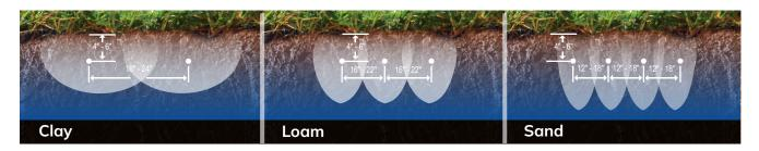
The following are cross-section views of a dripline row. These illustrations show water movement in a subsurface application. These guidelines apply to on-surface as well as subsurface installations.
